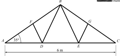
The length of [AC] is 6 metres, and the pitch of the roof is 35°, as shown. |AD| = |DE| = |EC| and |AF| = |FB| = |BG| = |GC|.
